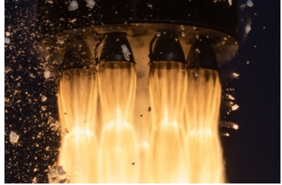
Electron's nine Rutherford engines during lift-off of the successful 'Return to Sender' first recovery mission (Rocket Lab)
